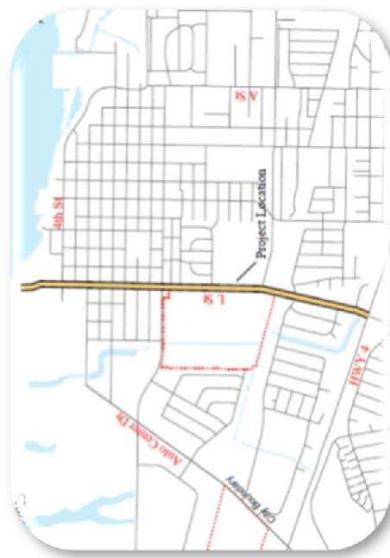
Project Description: This project will consist of modifying and widening portions of the roadway, constructing new concrete curb, gutter, sidewalks and curb cuts, installing landscaping and decorative hardscape, improve bicycle access and upgrading signage and striping throughout the project. The project will be constructed in 2 phases. Phase 1 is Hwy 4 to Sycamore and W 10th to Marina. Phase 2 is Sycamore to W 10th.
