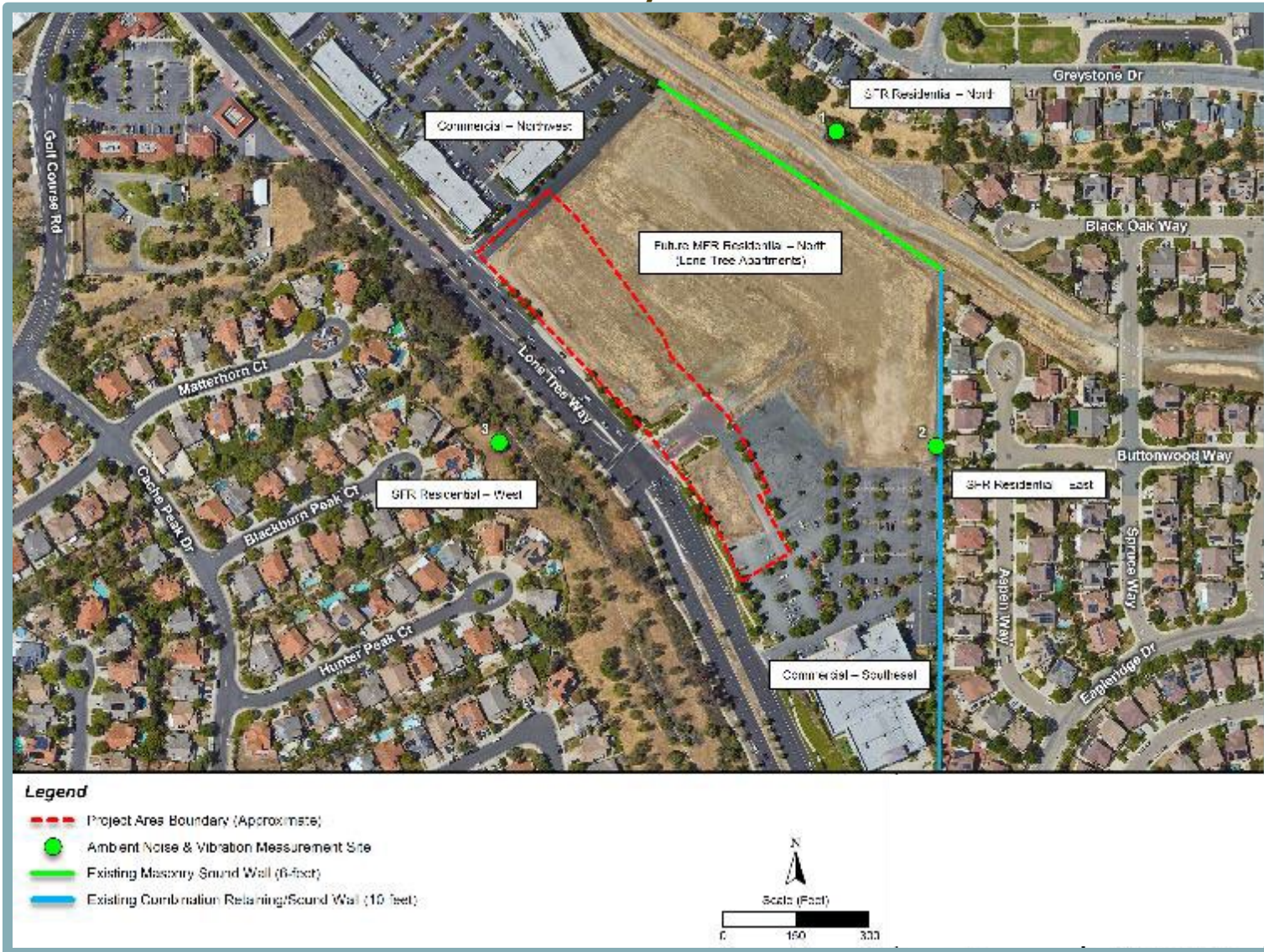
Figure 4 Noise Survey Locations
