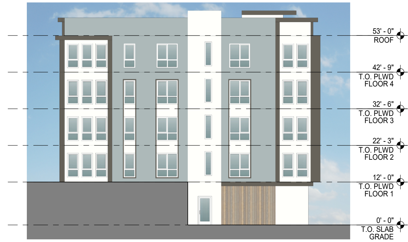
BUILDING D - WEST ELEVATION 4 1/16" = 1'-0"
