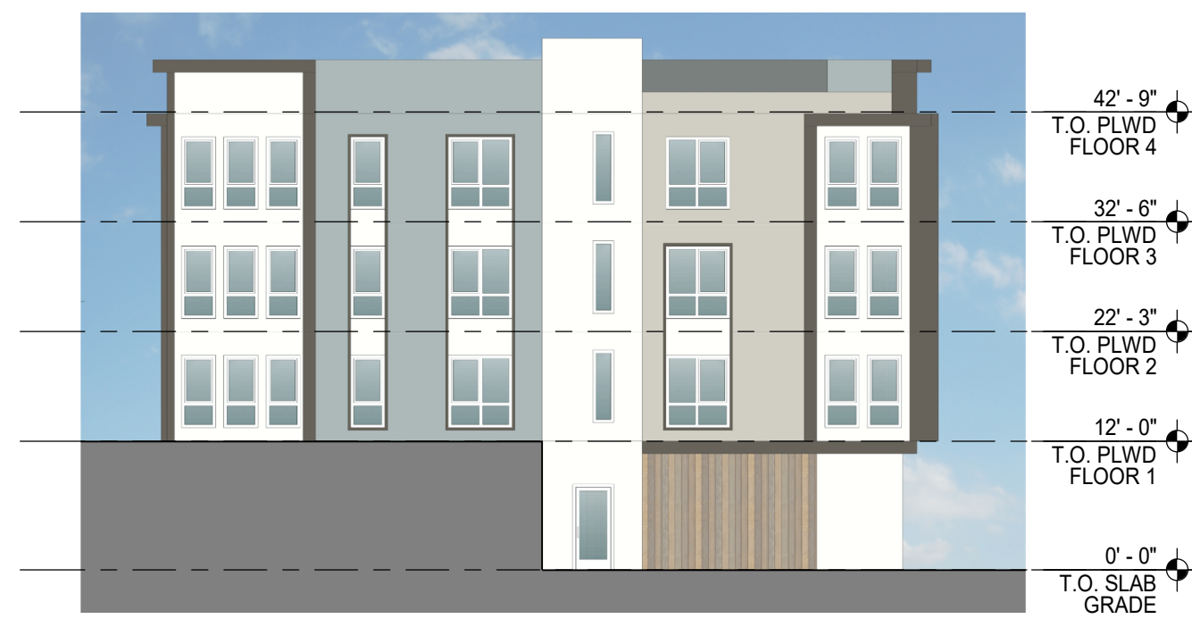
BUILDING B, C, F - WEST ELEVATION 8 1/16" = 1'-0"
