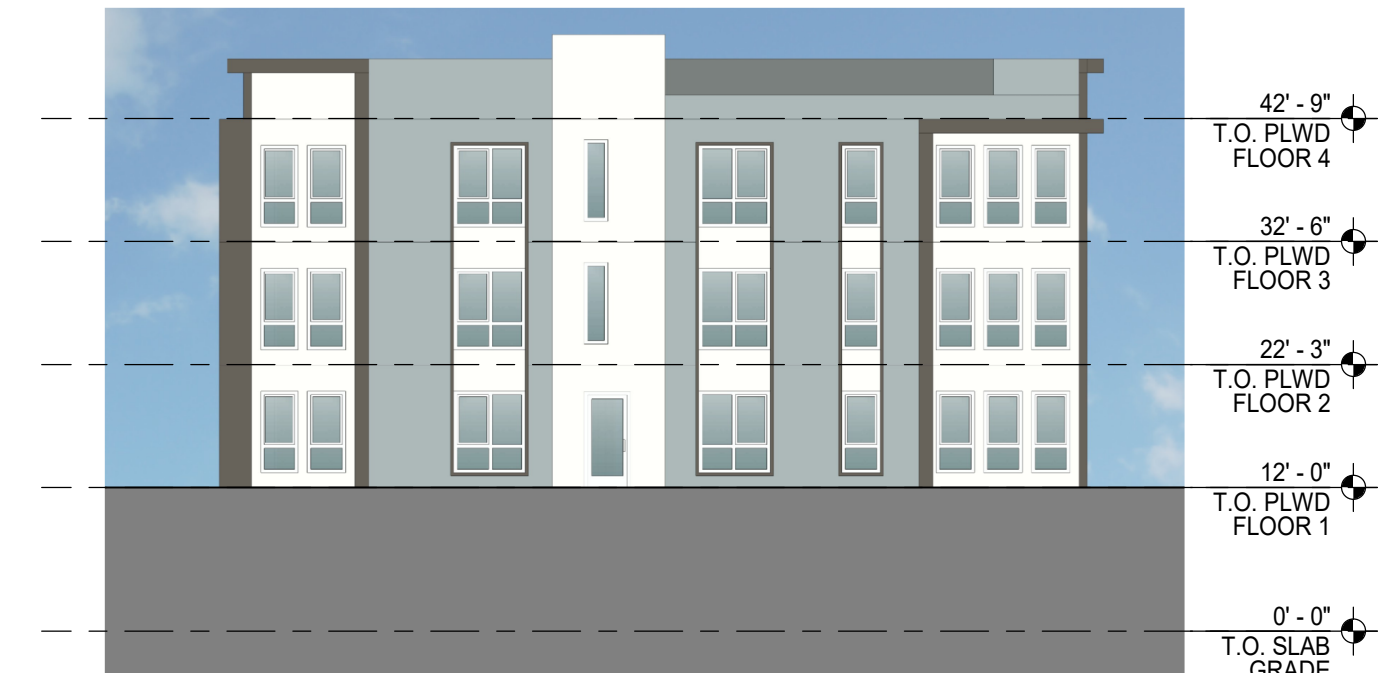
BUILDING A - SOUTH ELEVATION 3 1/16" = 1'-0"
