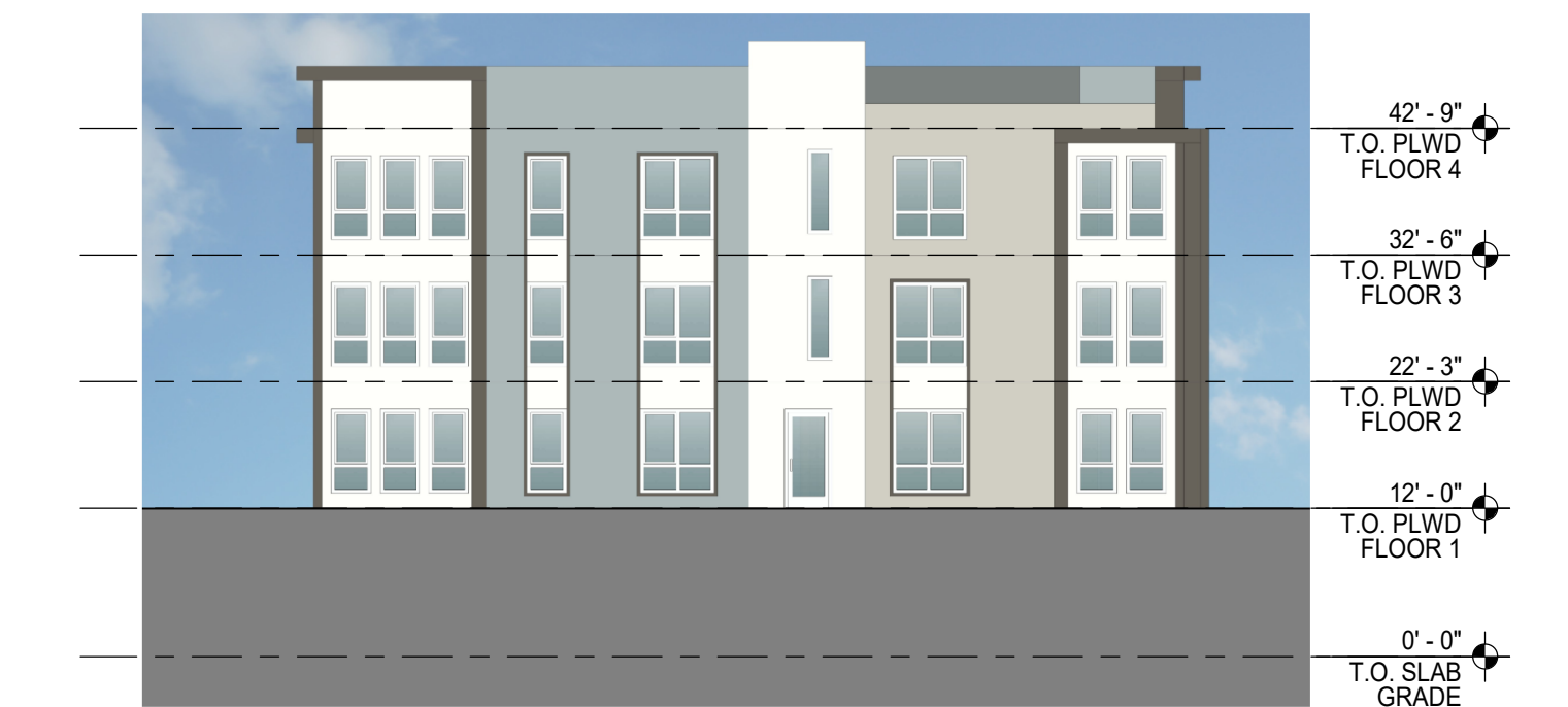
BUILDING A - NORTH ELEVATION 1 1/16" = 1'-0"
