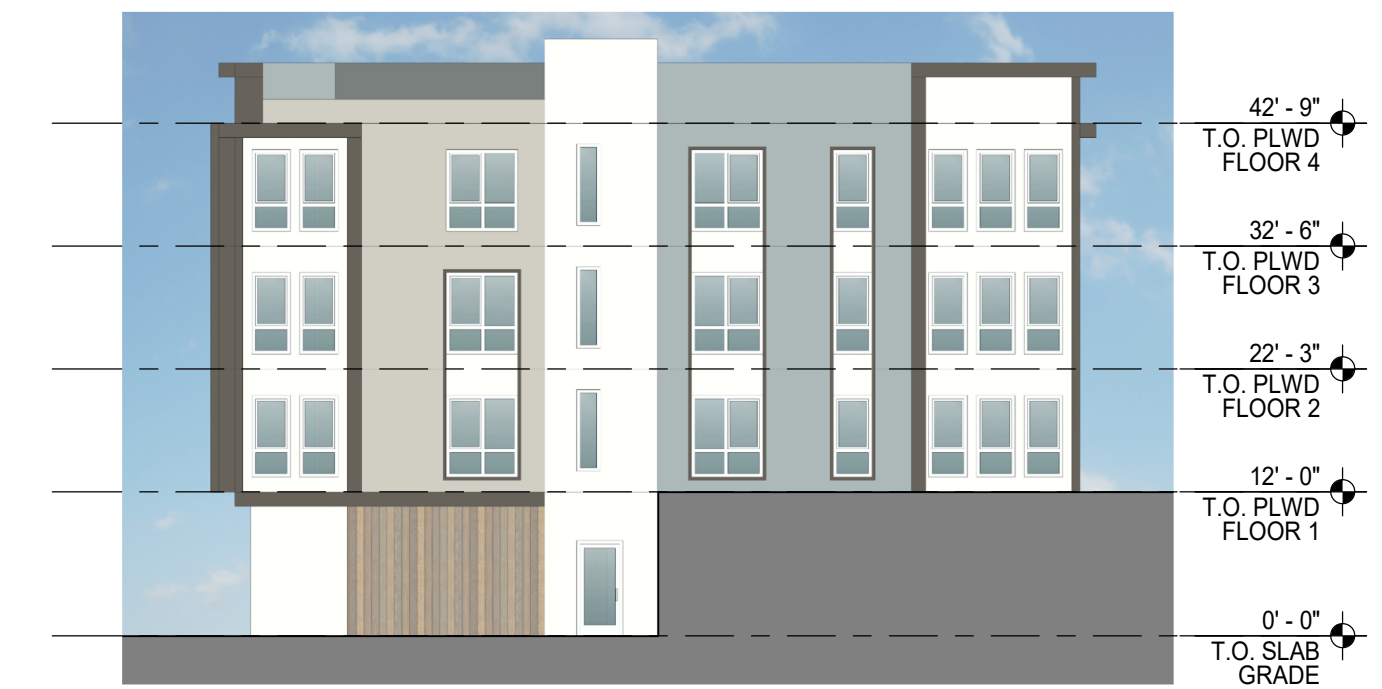
BUILDING E - EAST ELEVATION 2 1/16" = 1'-0"
